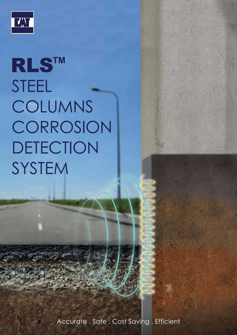
The RLS™ (Relative Loss of Section) system is a unique instrument that was specially developed in England to accurately quantify varying levels of corrosion around the entire mass of the critical zone of steel columns that cannot be identified by visual inspection, and provides precise recommendations for replacement or scheduling of subsequent testing.
